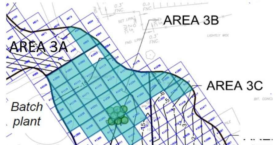
Note: Mixed areas indicated with blue shading. Green circles indicate previously-mixed field demonstration cell.
