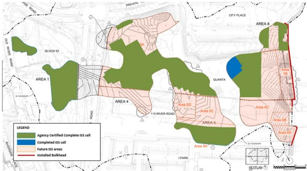
**Figure 1. Bulkhead and In Situ Solidification/Stabilization (ISS) Progress through December 2018**
