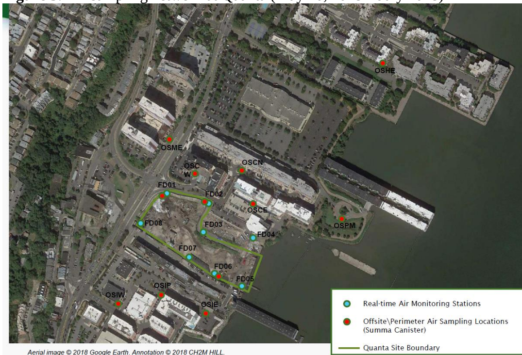
Figure 3: Air sampling network at Quanta (May 10, 2018 – July 2018)
