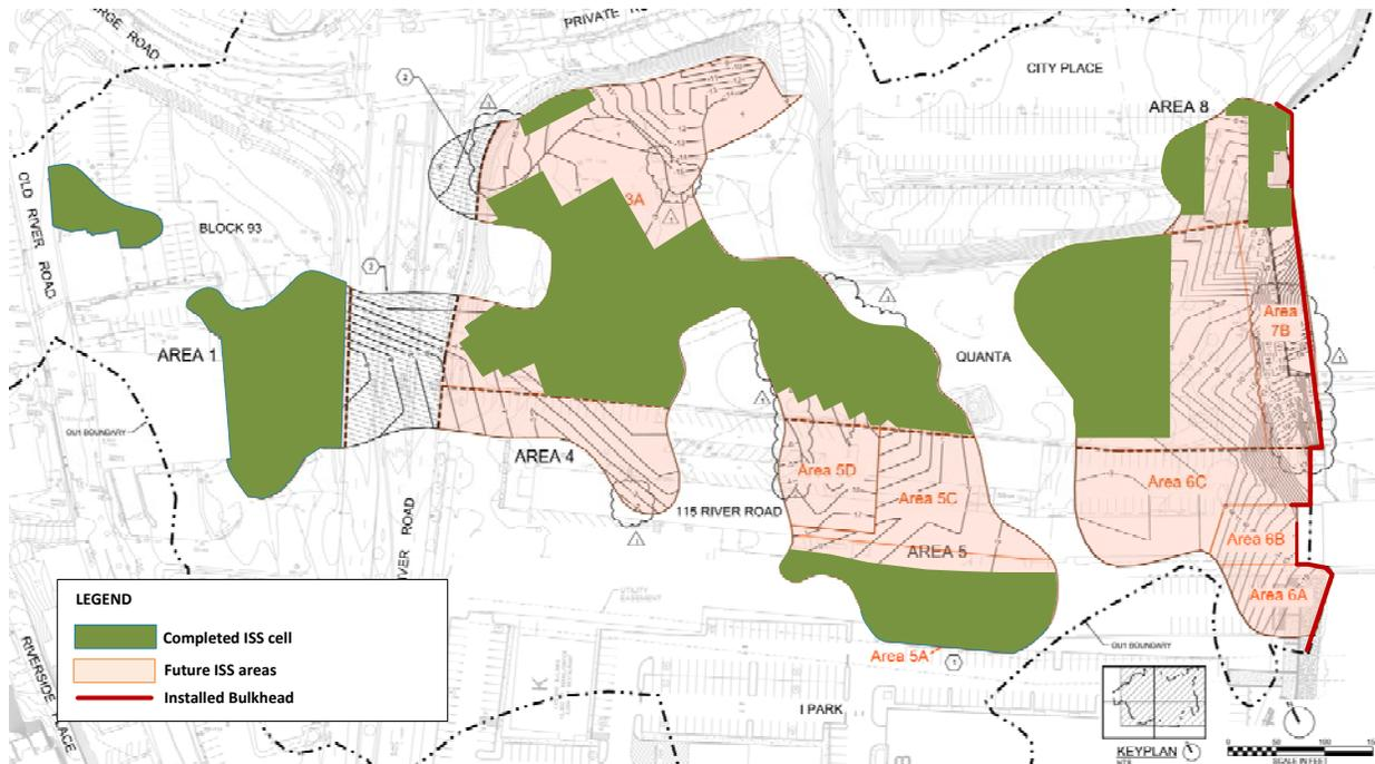
**Figure 1. Bulkhead and In Situ Solidification/Stabilization (ISS) Progress through May 2019**
